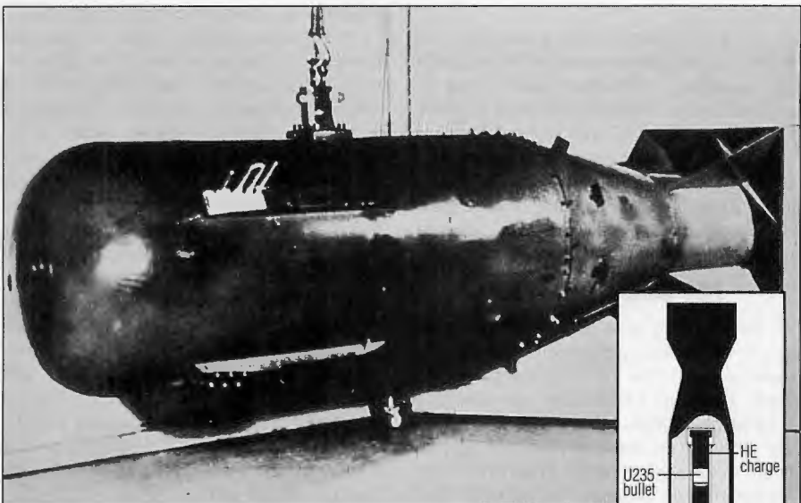
"Little Boy," the atomic bomb used at Hiroshima, was of the "gun-type" and weighed some 9,700 pounds. This is the type of bomb that Iran, 52 years later, is trying to build. (inset) The schematics of such a device are simple.
